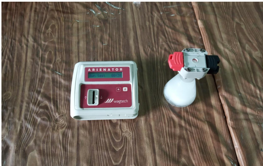
Figure 3.3: Arsenator set up for measuring arsenic concentrations
