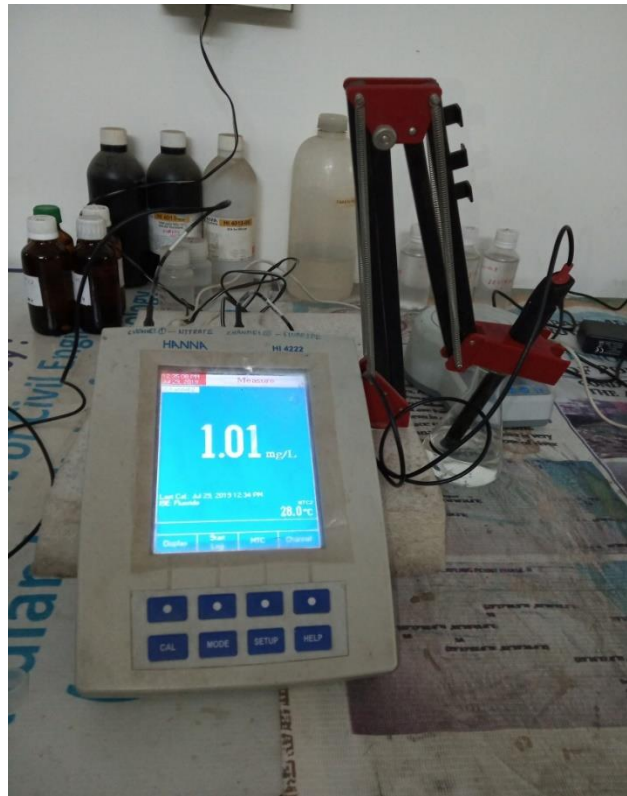
Figure 3.2: Ion meter for measuring nitrate and fluoride concentrations
