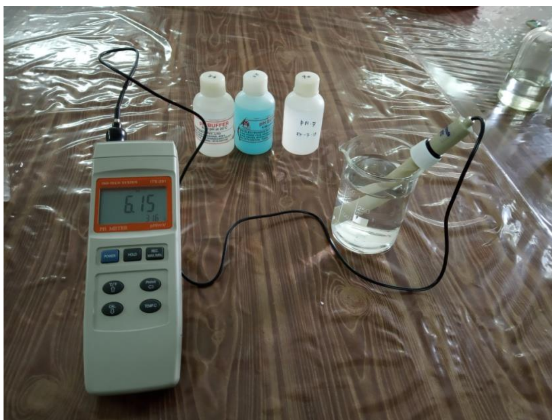
Figure 3.1: Ion meter for measuring pH
