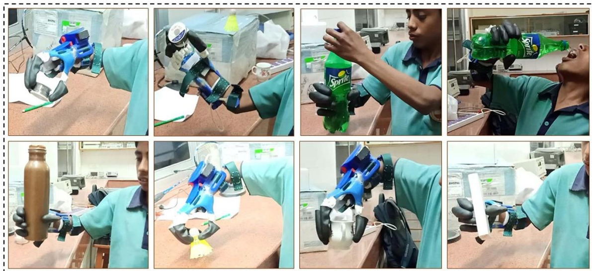
Figure 6.12 Activities performed by an amputee wearing the developed hand.
