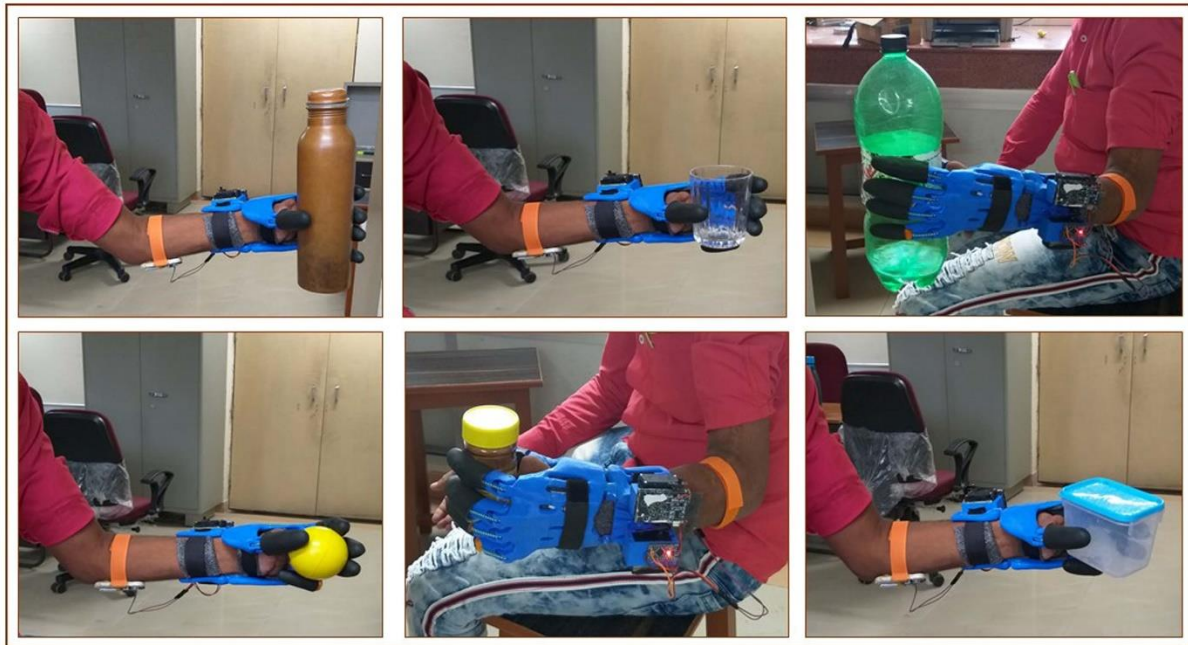
Figure 5.15 Different grasping operations performed by an amputee wearing a hand prosthesis.
