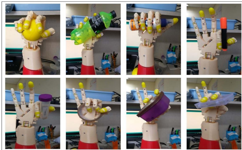
Figure 4.10 Different grasping actions performed by the prosthetic hand utilizing EMG signal from a subject.
