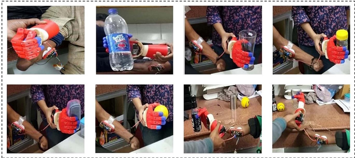
Figure 2.15 Performed operations by prosthetic hand using sEMG signal from amputees.
