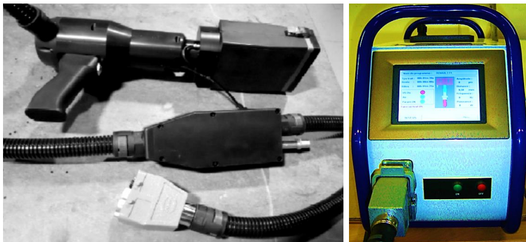
Fig. 2.1. The peening head (left) and the central unit (right) of the ultrasonic shot peening device.
