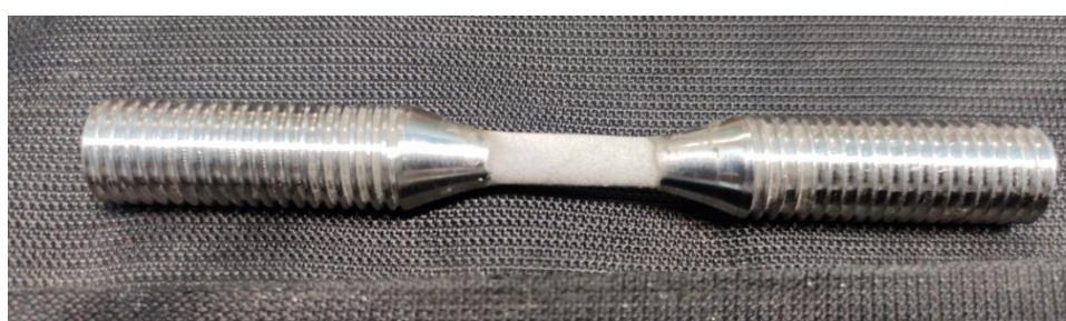
Fig. 2.9: Digital photograph of the LCF sample coated with thermal barrier coating.
