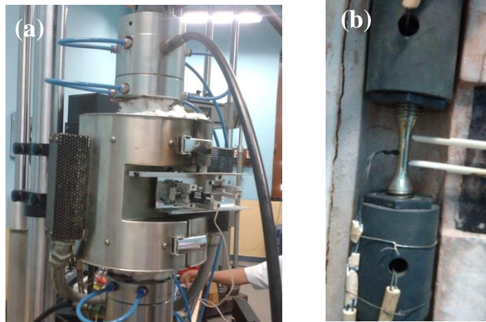
Fig. 2.4: (a) Machine set up for low cycle fatigue testing (Model: MTS 810) (b) High temperature extensometer and thermocouples mounted on the sample.
