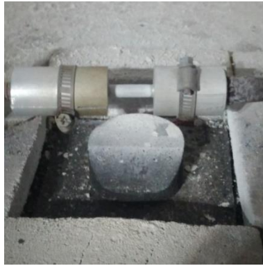
Fig. 2.6: Experimental set up for salt spray coating.
