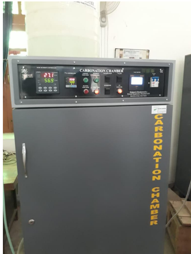
Fig 3.4 Preparation of Concrete Cubes and Placing of Samples in Carbonation Chamber- Departmental Laboratory, IIT (BHU), Varanasi
