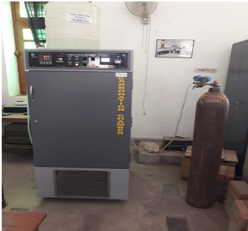
Fig 3.5 Carbonation Chamber - Departmental Laboratory, IIT (BHU), Varanasi
