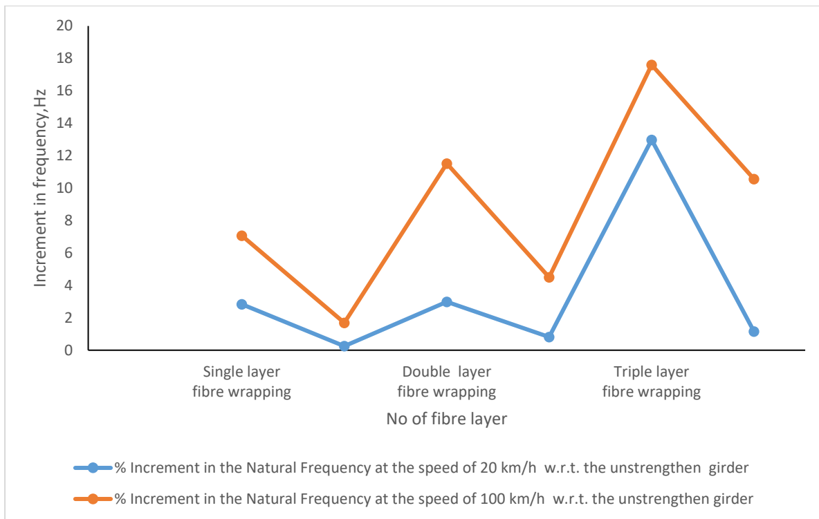
Figure 5. 49 Change in natural frequency at different fibre layer
