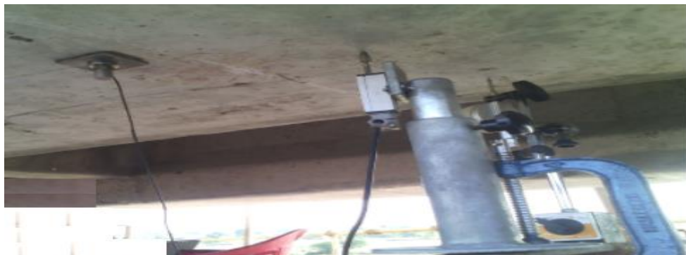
Figure 5. 41 Arrangement of deflection sensor and accelerometer
