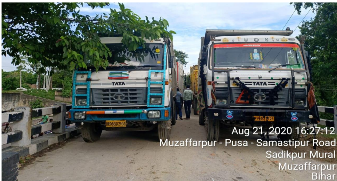
Figure 4. 46 Arrangement and axle load of four truck for case ii static load testing
