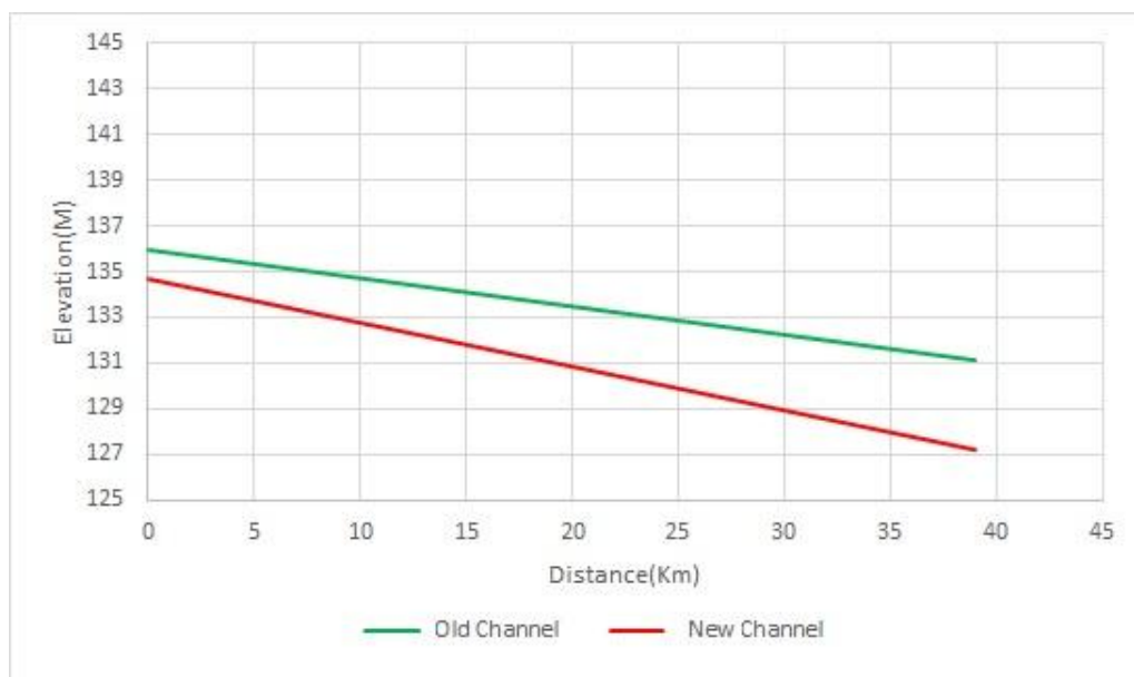
Figure 4.6 Longitudinal profile of a segment of Ramganga river of old (Gambhiri river) and new course (Kunda nala).
