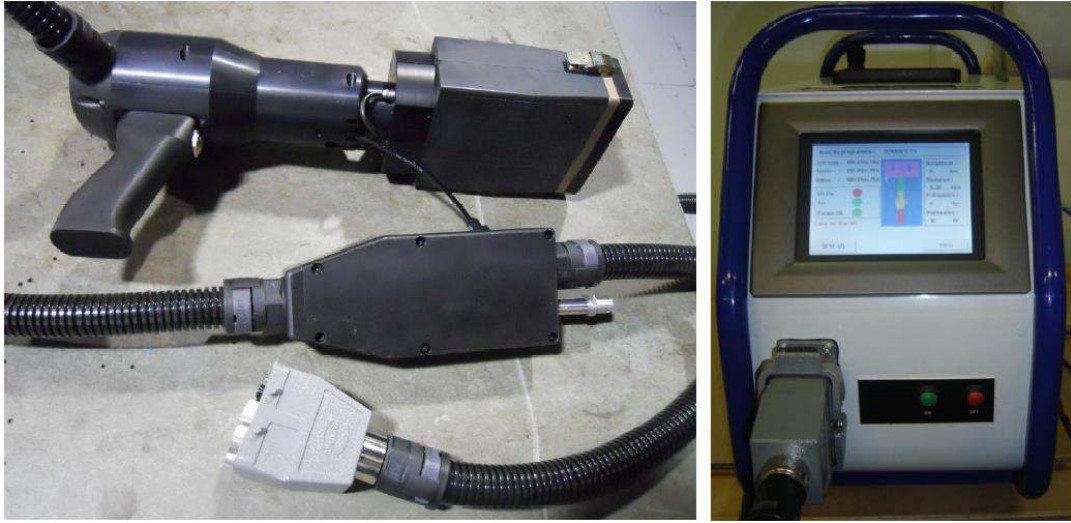
FIGURE 2.2: The peening head (left) and the central unit (right) of the ultrasonic shot peening device.
