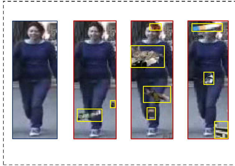
Figure 5.2: An original frame from the CUHK_03 data and the corresponding occluded frames generated by adding varying degrees of synthetic occlusion
