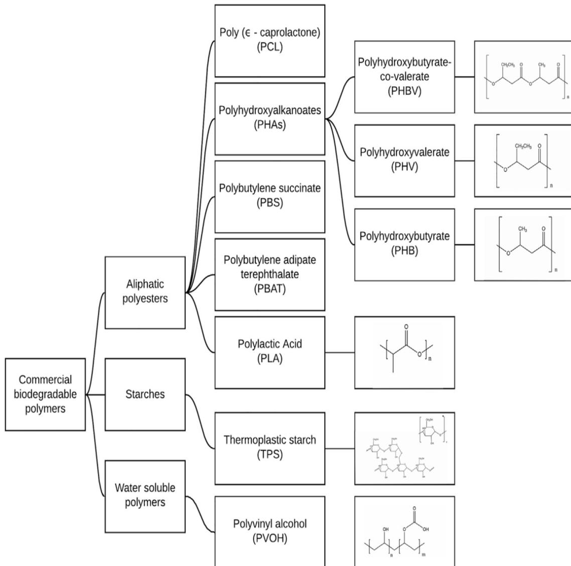
Figure 1.1: Commercial biodegradable thermoplastics [5]
