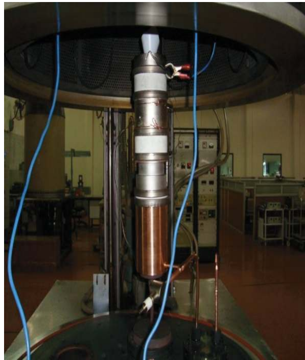
Fig. 3.11: Vacuum processing of MIG at BEL, Bangalore.
