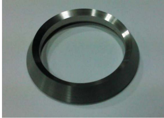
Fig. 3.7: Cathode pellet procured from M/S Semicon, US.
