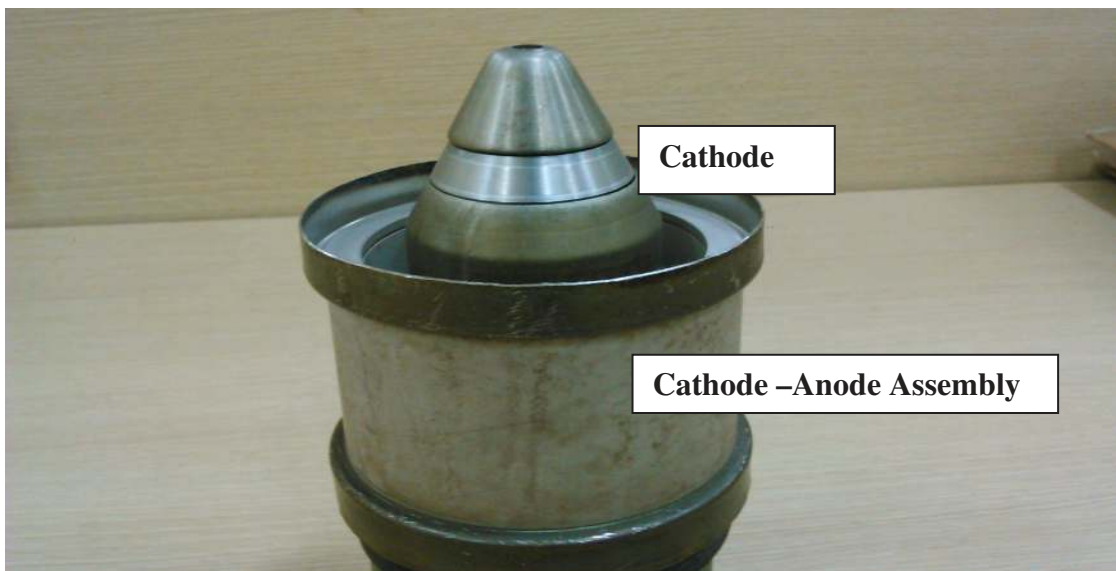
Fig 2.10: Cathode assembled with modulating anode
