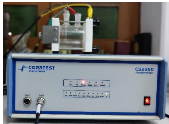
Figure 2.6: Photograph of CorrTest electrochemical work station, with flat type corrosion cell.
