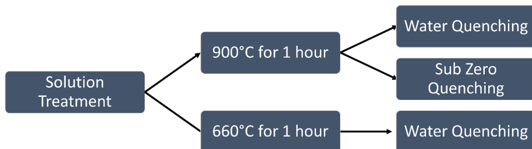
Figure 3.1 Heat treatment outline for the alloy Ti-13Nb-13Zr.
