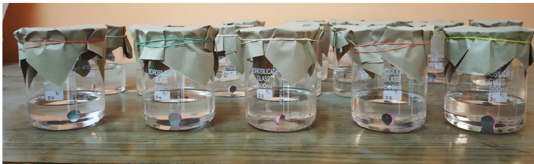
Figure 2.5 Test samples suspended in Ringer's solution for static immersion test.
