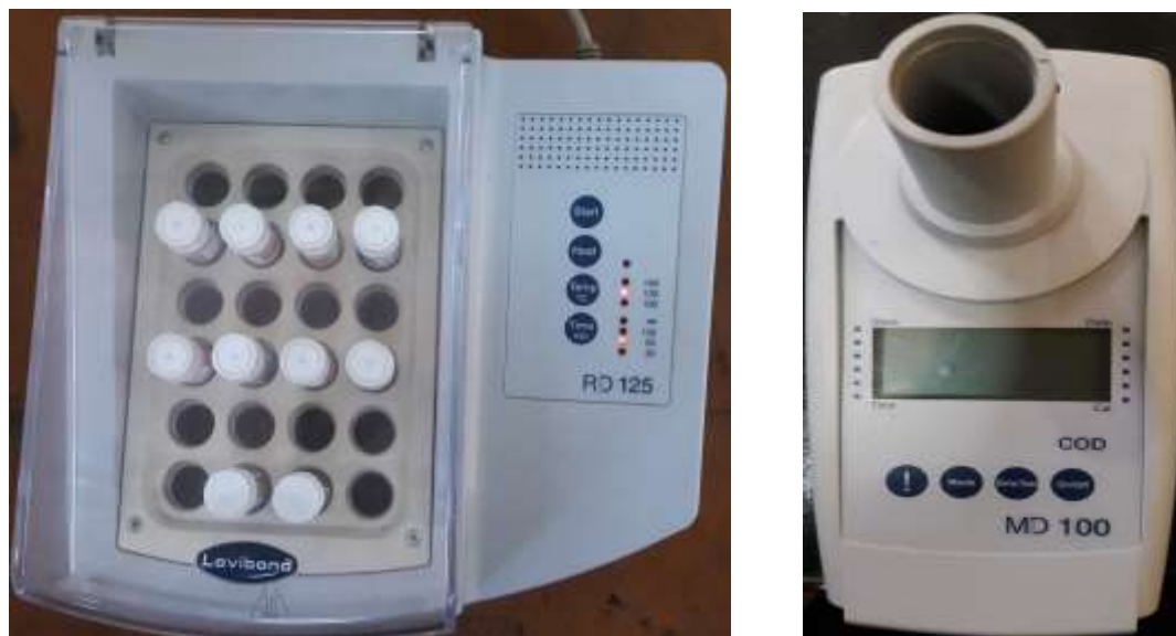
Figure 5.7: Digester and photometer for COD measurement.
