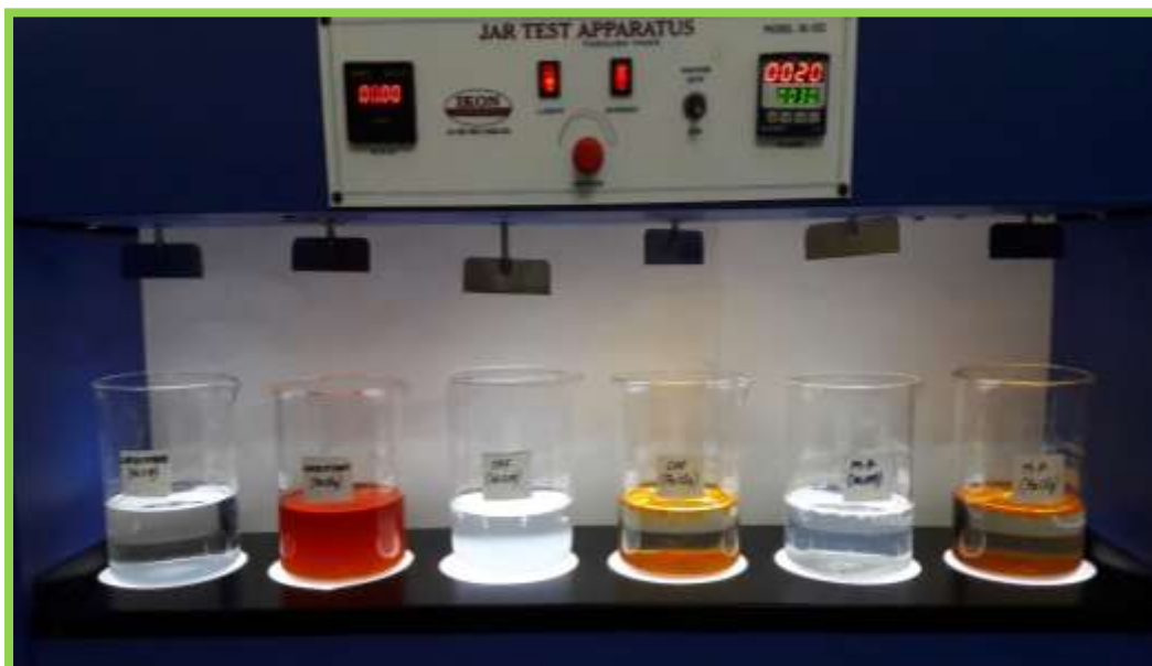
Figure 5.3: Jar-test apparatus for coagulation-flocculation process.
