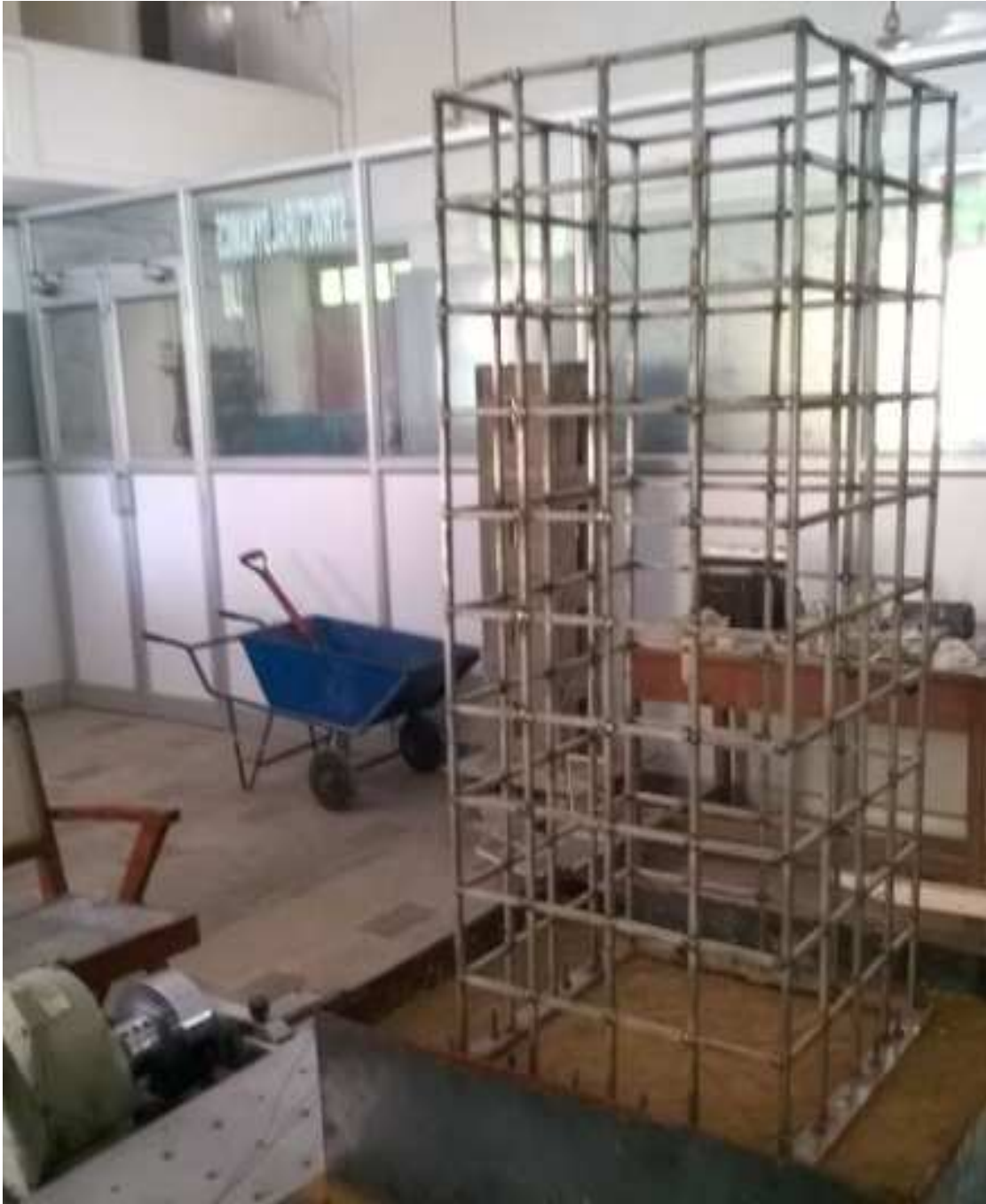
(b) Model with base fix in soil Fig.7.2. Model with fixed base and with base fix in soil
