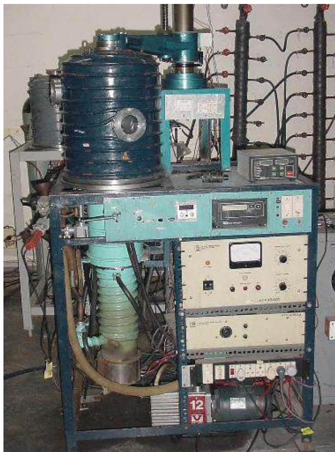
Fig.3.7 Electron beam evaporation unit used for the deposition of \text{TiO}_2 film.
