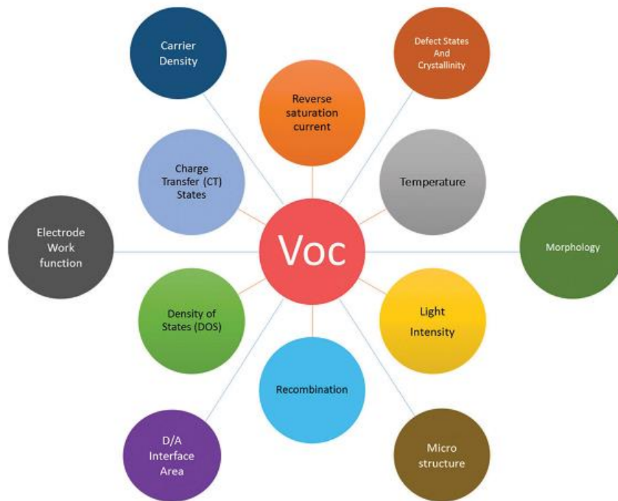
Figure 1.12: Factors influencing the open-circuit voltage in OPV [40].
