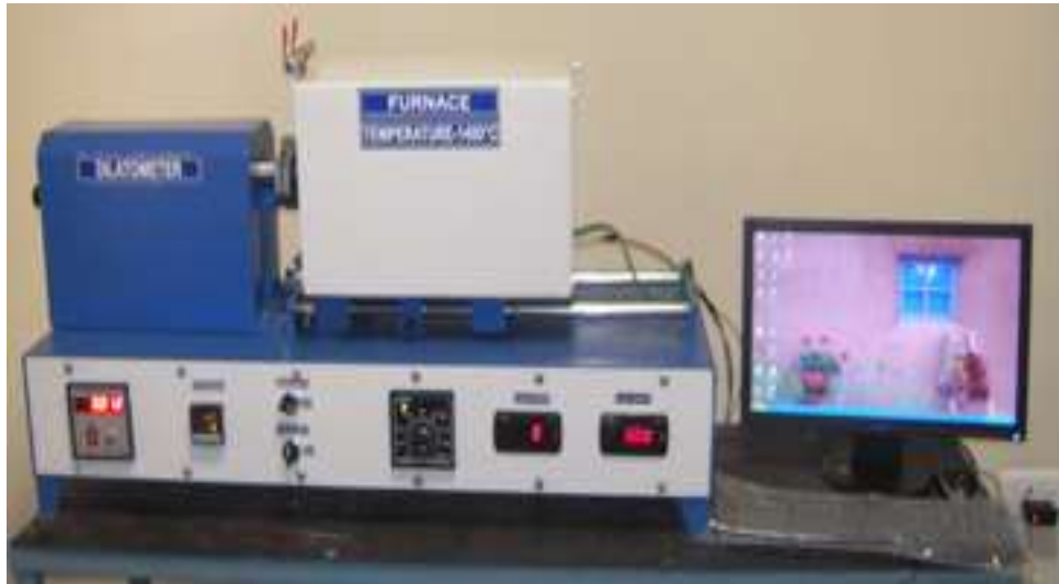
Fig. 3.7 Image of pushrod dilatometer [ http// www.vbceramics.com ]
