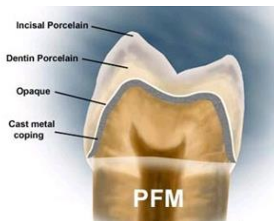
Fig.1.1 a schematic image of metal ceramic crown [http://www.nobledental.com.au]
