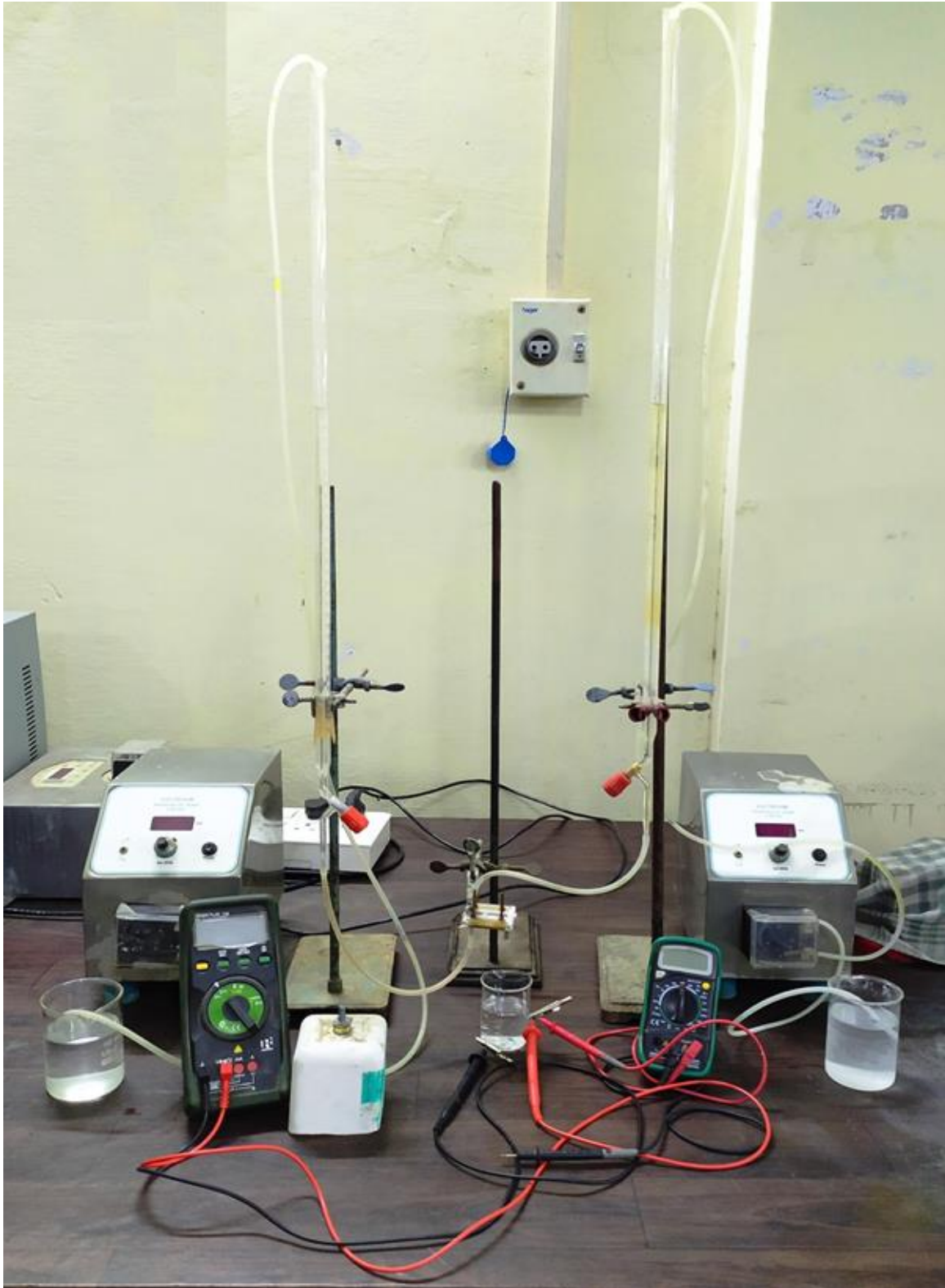
Figure A2 Photographic view of the air breathing T-shaped MFC experimental setup.
