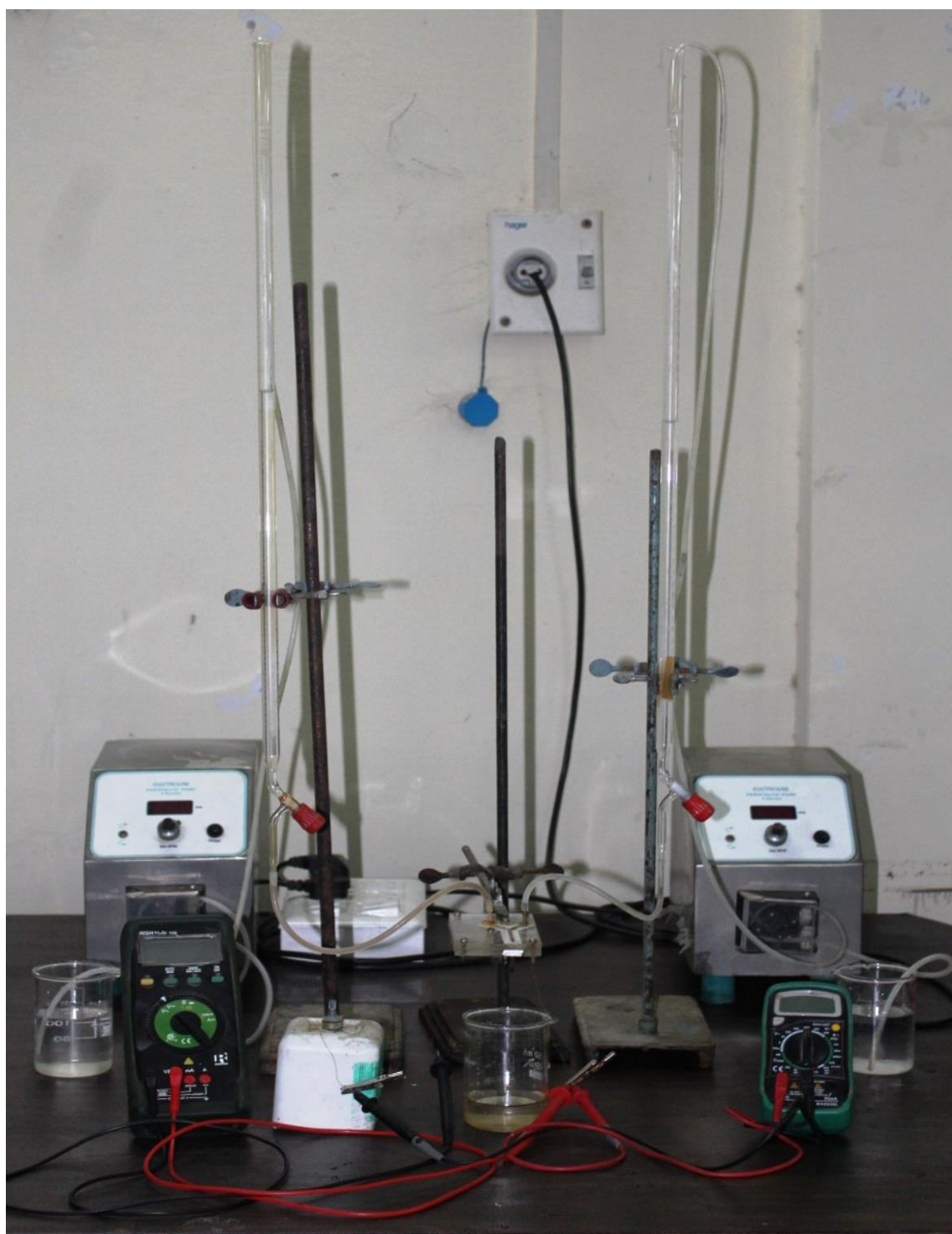
Figure A1 Photographic view of the air breathing Y-shaped MFC experimental setup.
