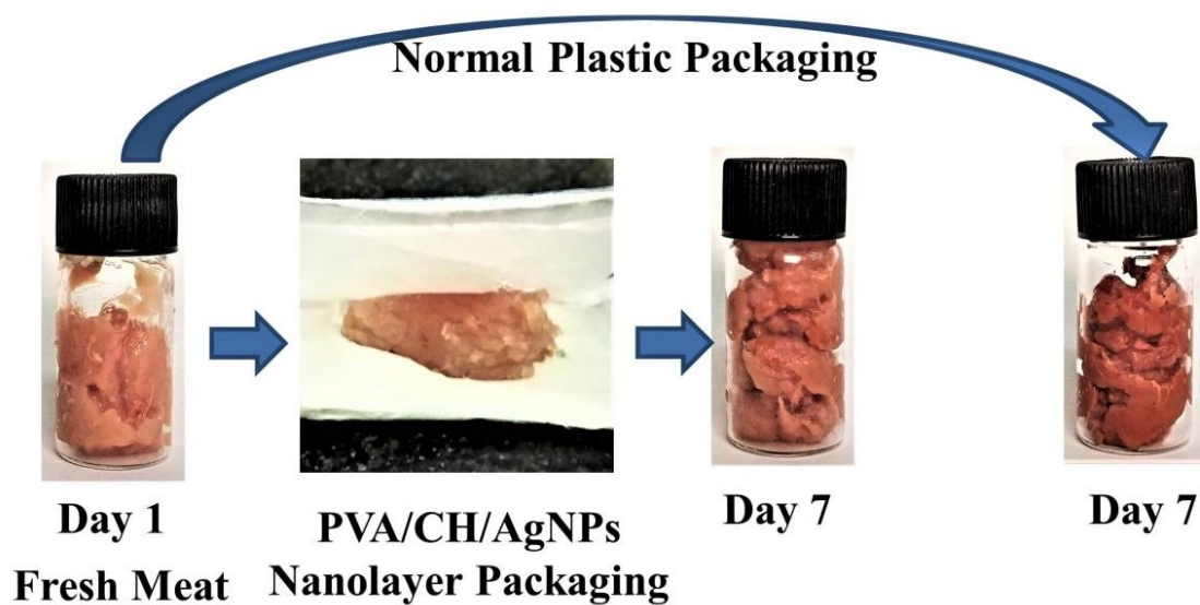
Figure 2.17: Application of PVA/CH/AgNPs composite nano-layer for packaging of fresh meat
