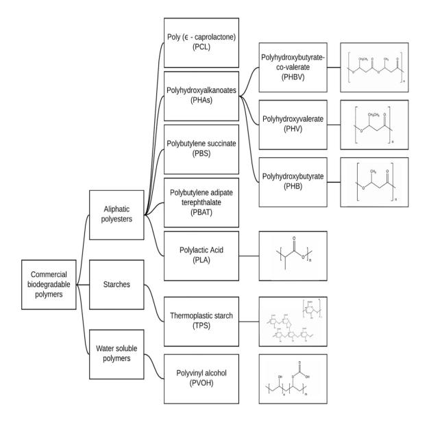
Figure 1.1: Commercial biodegradable thermoplastics [5]
