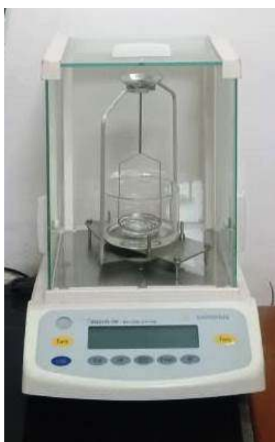
Figure 2.7: The density measurement kit (Denver SI-234).
