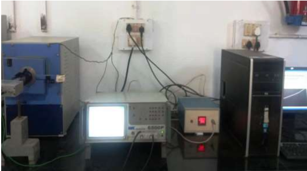
Figure 2.11: Computer controlled automated impedance analyser setup along with sample holder and furnace (6500 P Wayne Kerr, UK).
