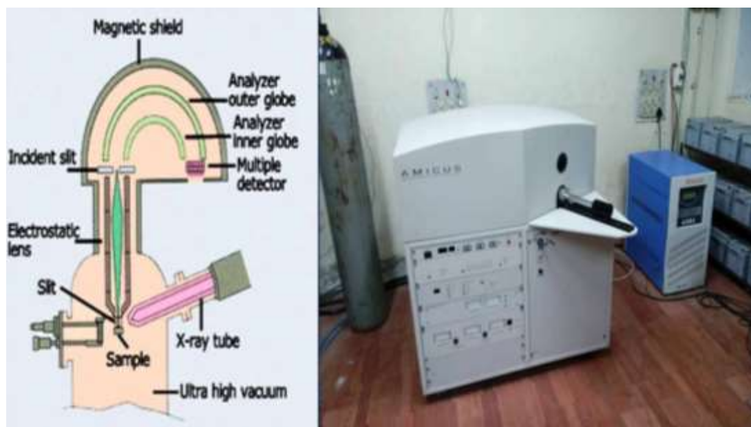
Figure 2.10: A Schematic design of XPS (X-ray photoelectron spectroscopy) working with photograph of XPS setup (KRATOS Amicus model).
