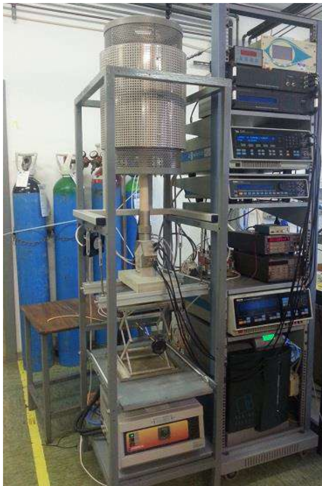
Figure 2.12: The Probostat (Norecs, Norway) system impedance Analyser (FRA, mod. SOLARTRON 1250 - Schlumberger), in a range of frequency between 1-10^6 Hz.
