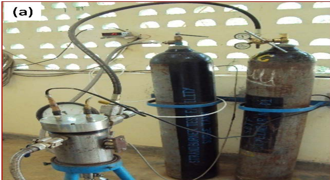
Fig.3.9: Photograph of Crawford Bomb for Burn Rate Measurement
