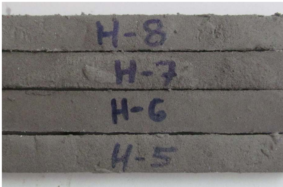
Fig 3.6. Samples of AP Based Solid Composite Propellant
