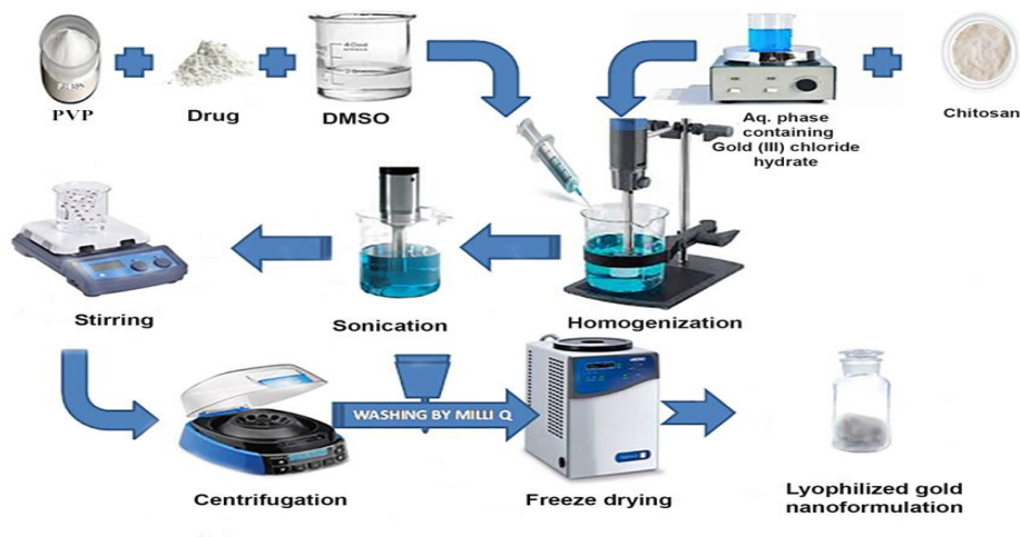
Figure 4.1 Preparation of DSB loaded PVP stabilized chitosan capped gold nanoparticles
