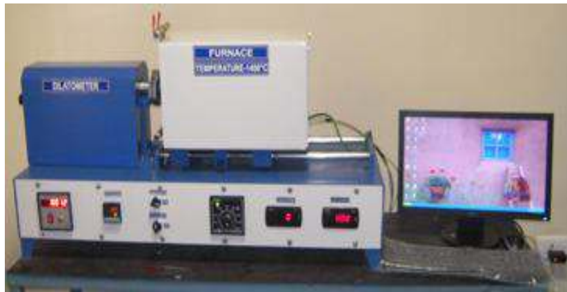
Fig. 3.9 Image of pushrod dilatometer [www.vbceramics.com]
