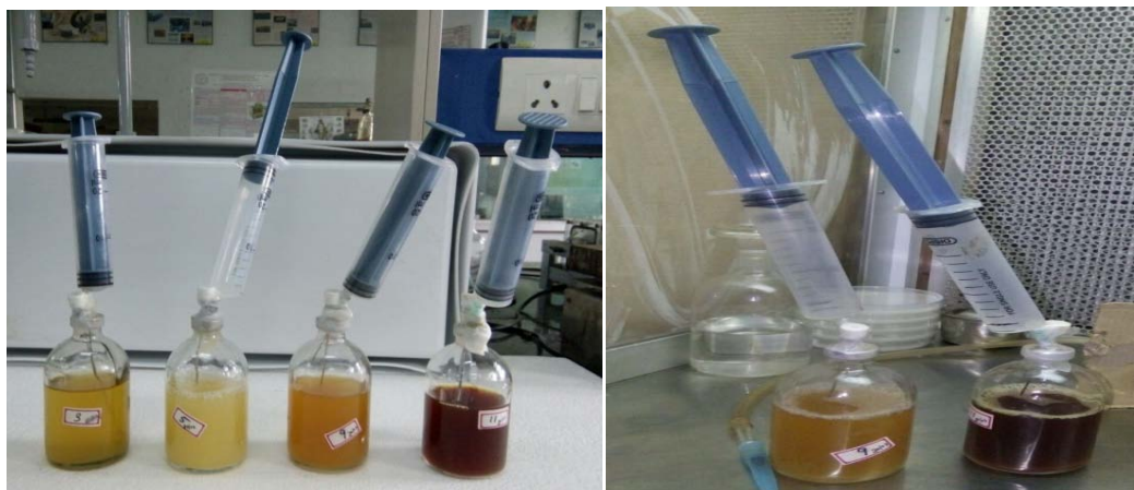
Figure 4.23: Serum bottles with crimped cap for anaerobic fermentation study
