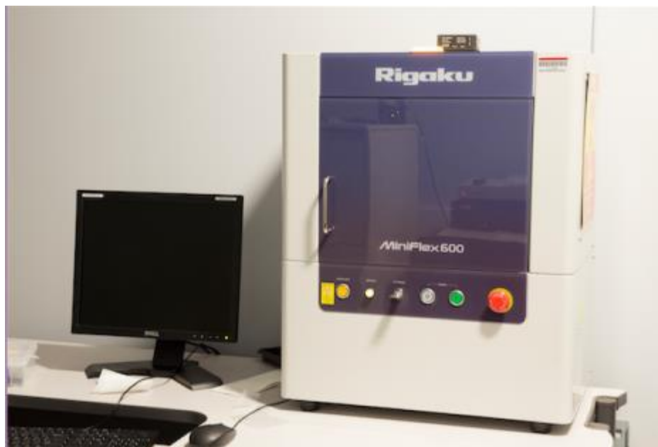
Figure 2.2 Powder XRD instrument, Rigaku Miniflex 600 (Japan)
