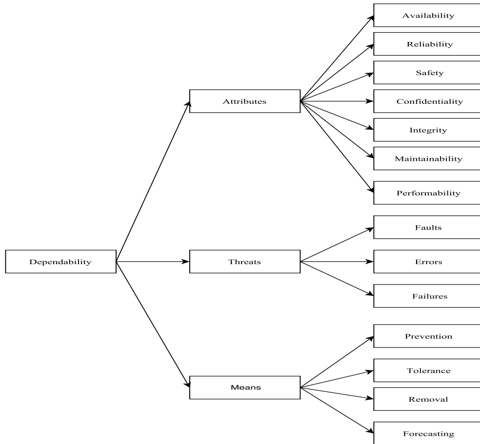
FIGURE 1.1: Taxonomy showing relationship between Dependability and Attributes, Threats and Means (after Laprie et al.)
