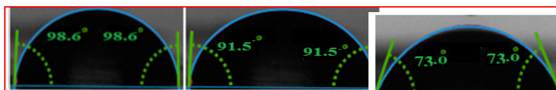
Fig.5.6 Contact angle of blank (a), thermally treated (b) and biodegraded (c) LDPE film
