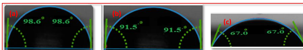
Fig.4.6 Contact angle of blank LDPE (a), thermally treated LDPE (b) and biologically treated LDPE film (c)
