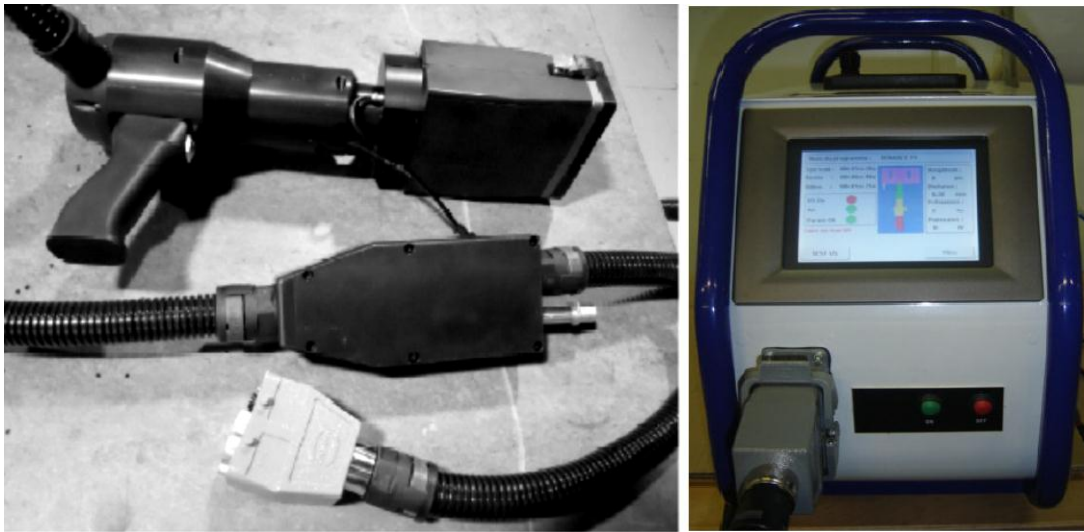
Fig. 2.1 The peening head (left) and the central unit (right) of the ultrasonic shot peening device.
