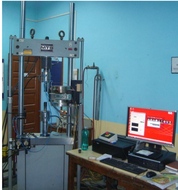
Fig. 2.4 Servohydraulic MTS for fatigue testing.
