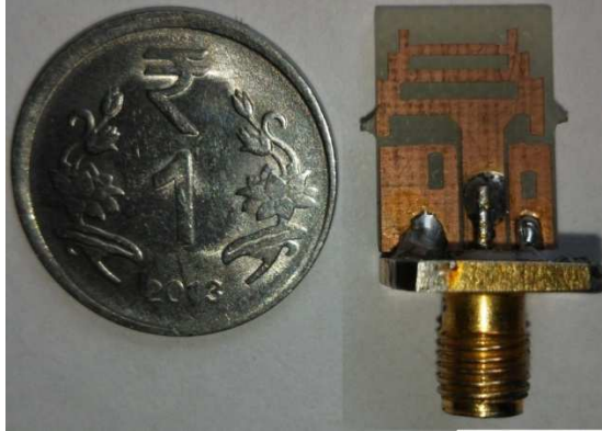
Figure 3.6 Prototype of the ladder shaped fractal antenna
