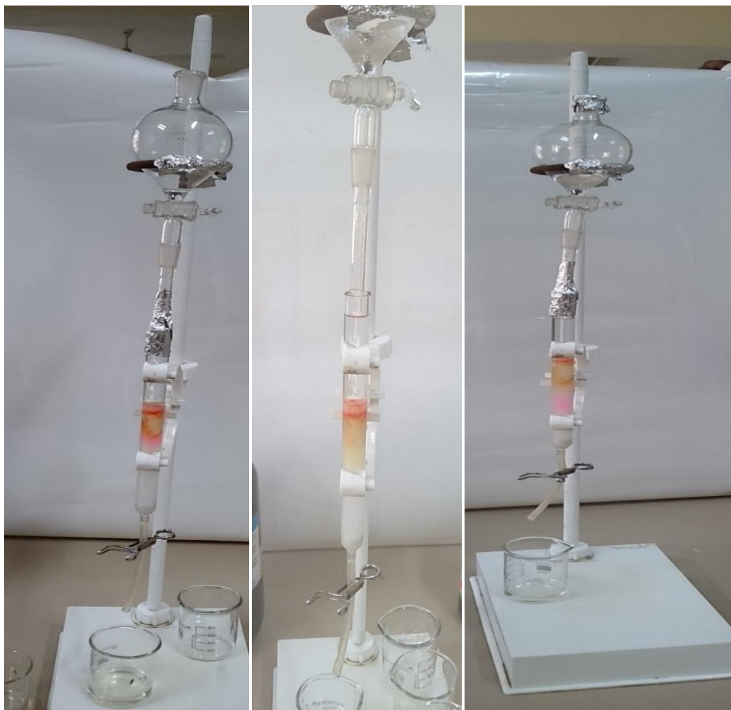
Figure 3.4: Different stages of column chromatography during fractionation of crude metabolite.
