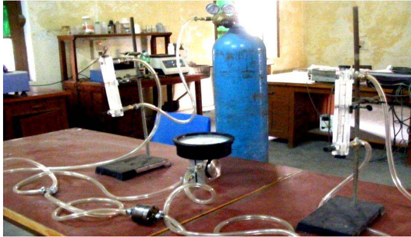
Fig. 9.2 Set up for measurement of gas permeability of porous ceramics
