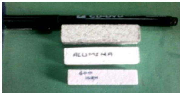
Fig. 5.10 Sample Al 420-600 RH 10 before and after firing
