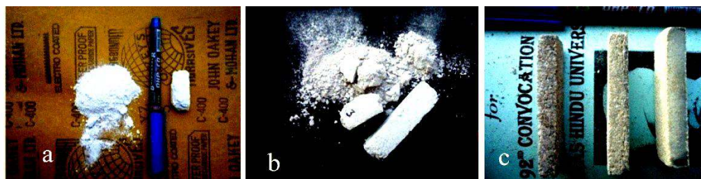
Fig. 5.7 (a) Cracking and bending in samples with 30 and 40 wt%, (b) Bursting of 30 wt% RH sample into powder after drying at 100 °C/24 h and (c) alumina samples with 10 and 20 wt% RH heated at 5 °C/min
