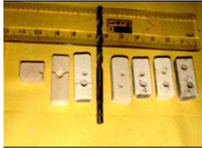
Fig. 4.4 Drilled green alumina samples prepared with sucrose content 1.8, 2.4, 3, wt% (left) and 3.6, 4.8, 6, 7.2 wt% (right)
