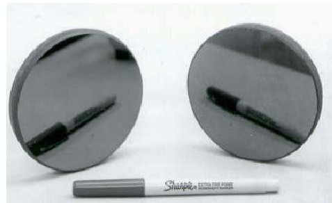
Fig. 1.4 Light weight space mirrors with porous SiC used as a support for dense polished SiC reflecting layer 207
