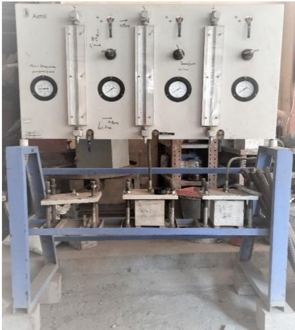
Figure 2. Water permeability setup
