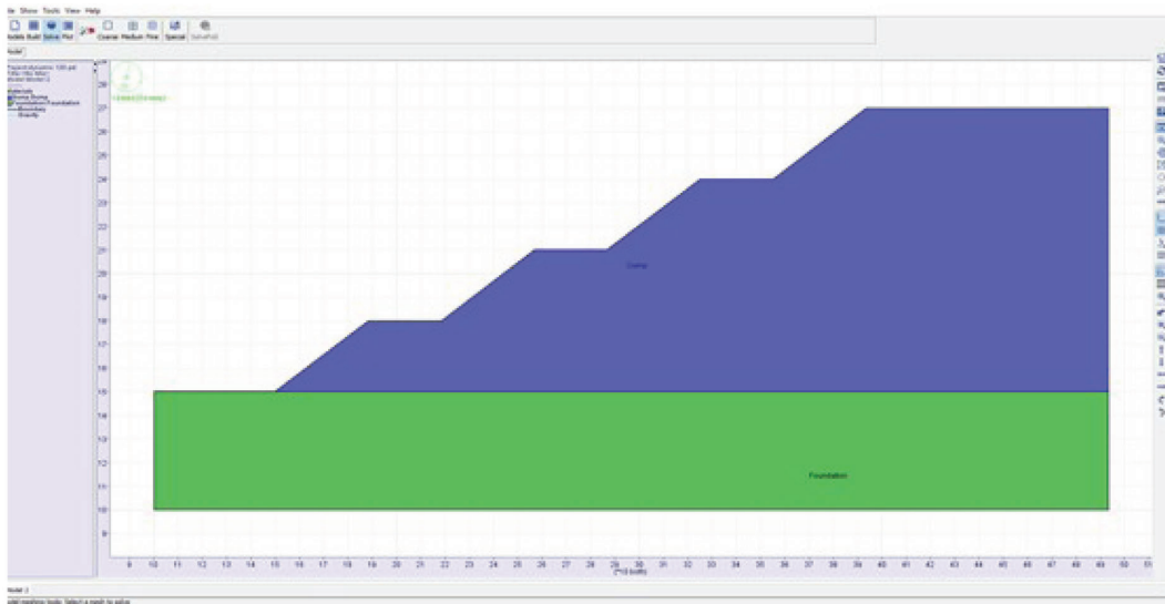
Figure 4. Dump model subjected to seismic loading along the X- and Y-axes.
