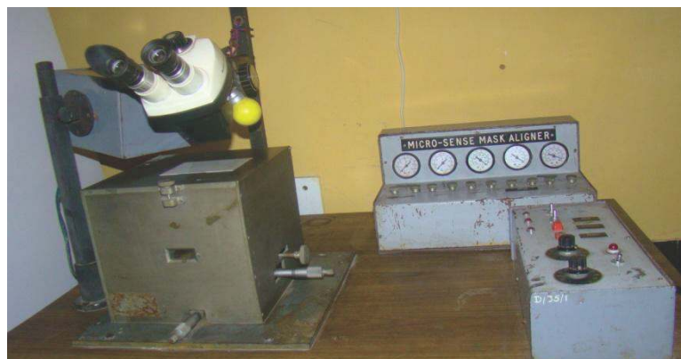
Plate 3.4: Photolithography Set-up (a) Spin Coater (b) Set-up for UV exposure
