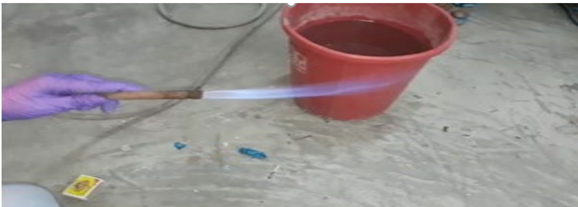
Fig. 3 Flame of hydrogen- and methane-rich produced gas from the stepped pyrolysis of biomass
