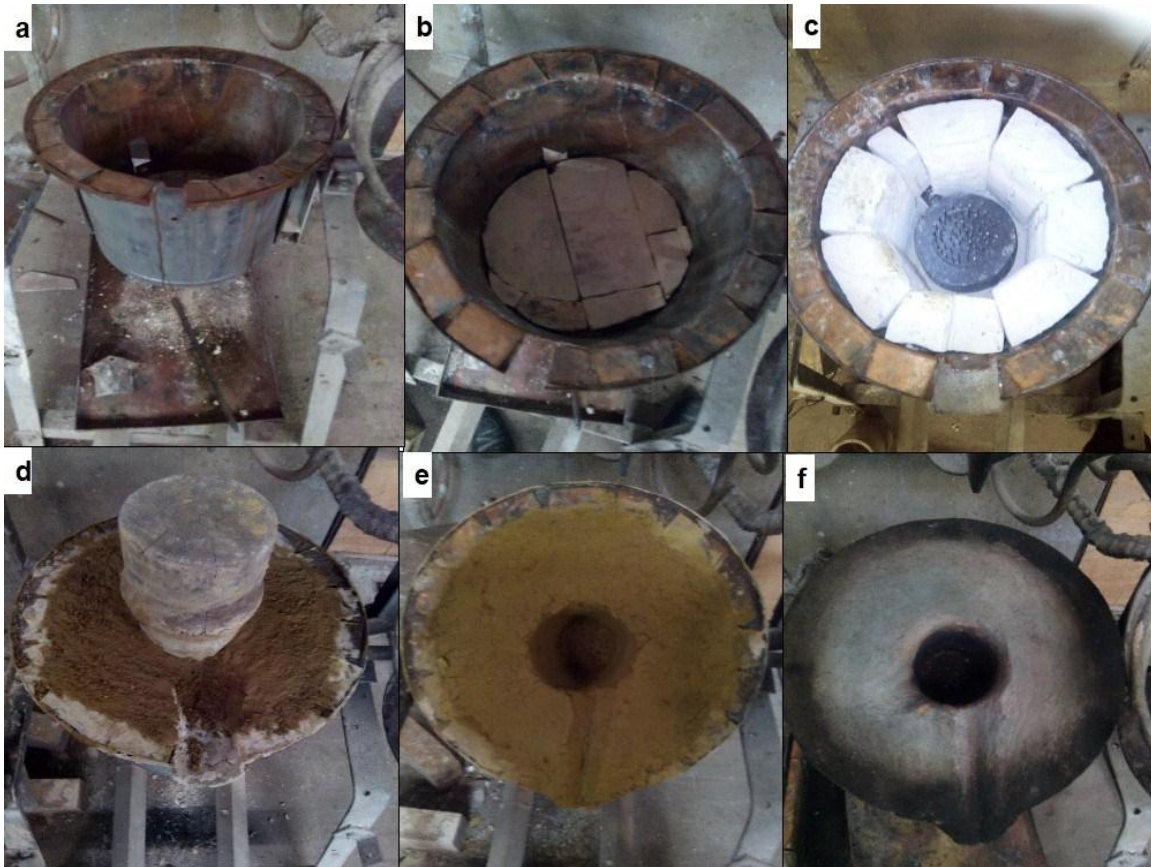
Figure 5. 4 Steps of making magnesite crucible
