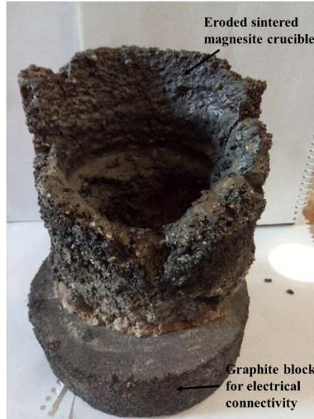
Figure 5. 22 Photograph shows the condition of sintered crucible after using 7 heats in nitrogen plasma
