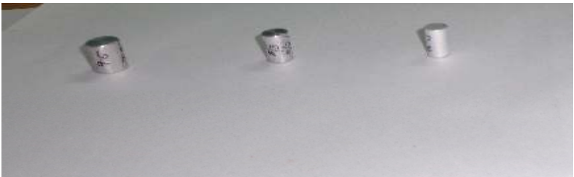
Figure 5.16: Microstructure samples of Aluminum rod before and after extrusion
