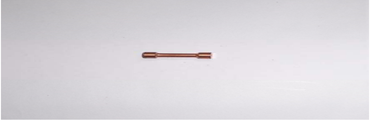
Figure 5.38: Tensile sample of extruded Copper rod (Gauge Length=15.6 mm, Gauge diameter = 4.5 mm)
