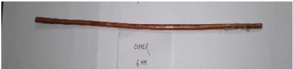
Figure 5.9: Extruded Copper product (6 mm diameter at 6RPM, extrusion ratio 4.34)
