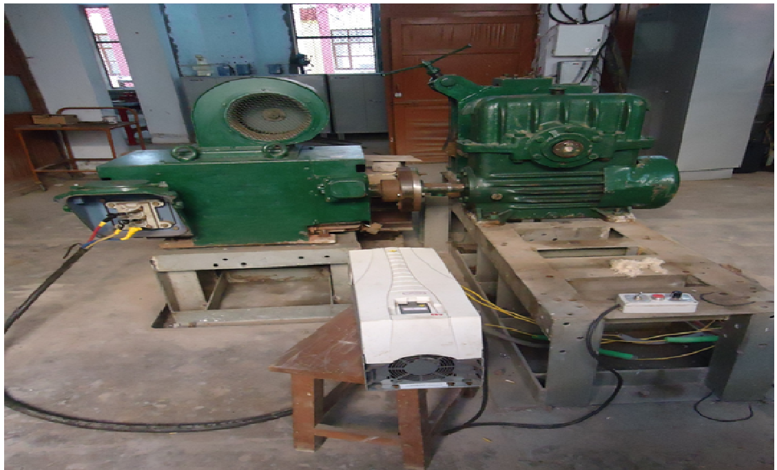
Figure 5.2: Fabricated Continuous Extrusion setup 2 (9.5 mm Aluminum feedstock material)
