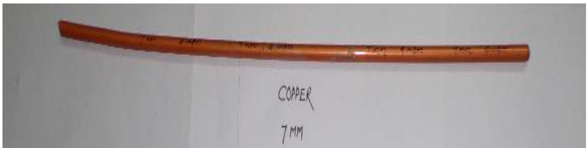
Figure 5.10: Extruded Copper rod (7mm diameter at 6 RPM, extrusion ratio 3.18)
