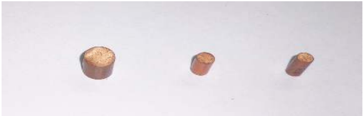
Figure 5.41: Hardness test samples of Copper rod before and after extrusion
