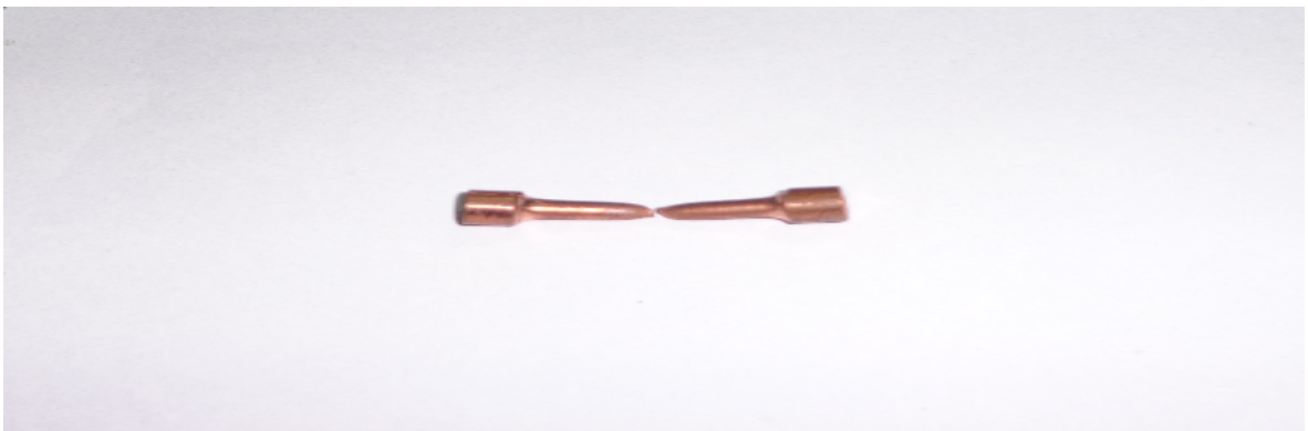
Figure 5.39: Fractured tensile sample of extruded Copper rod
